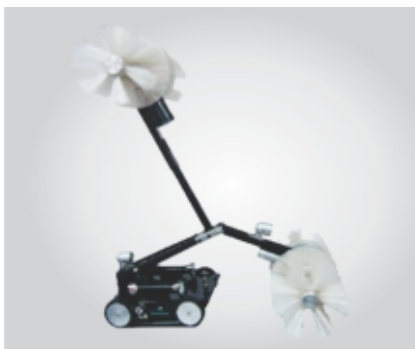
NBB, Brushing And Suction Robot Duct Size Upto 5 feet
